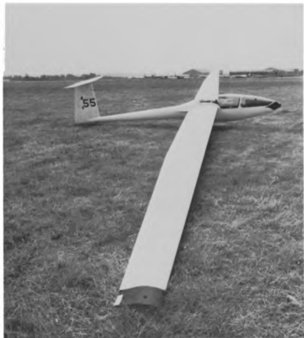
6 The Libelle. A new era of glider construction began when glass-reinforced plastics, more commonly called fibreglass, were introduced. The advantage of these materials is the high standard of surface finish which can be achieved. This Libelle has a span of fifteen metres and a best glide angle of one in thirty-eight
