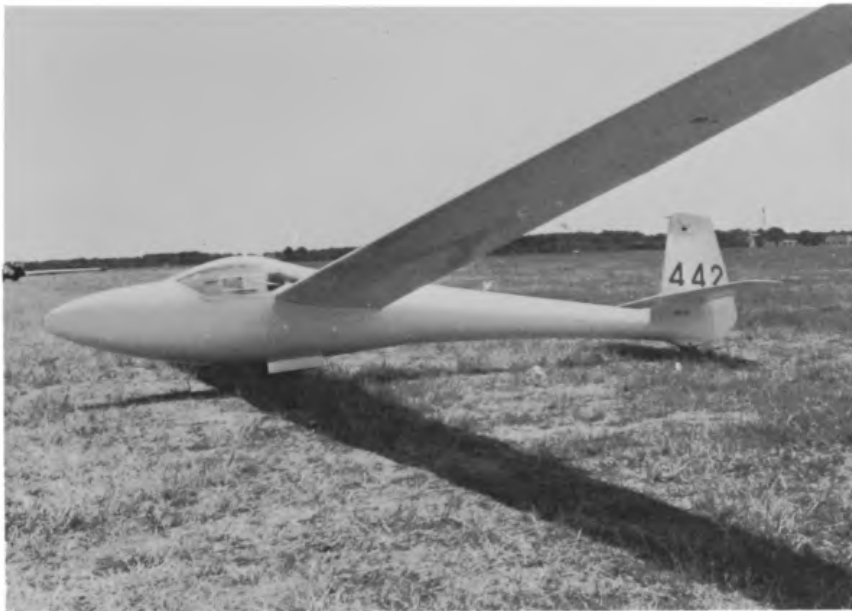
6 The Libelle. A new era of glider construction began when glass-reinforced plastics, more commonly called fibreglass, were introduced. The advantage of these materials is the high standard of surface finish which can be achieved. This Libelle has a span of fifteen metres and a best glide angle of one in thirty-eight
